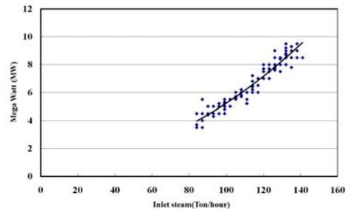
Fig. 2. Electric Power Curve of Turbo Generator based on Changes of Steam Mass
