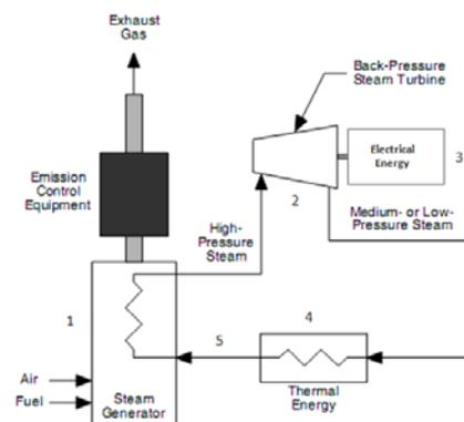
Fig. 1. Schematic performance of CHP System based on back-pressure Steam turbine [3]
