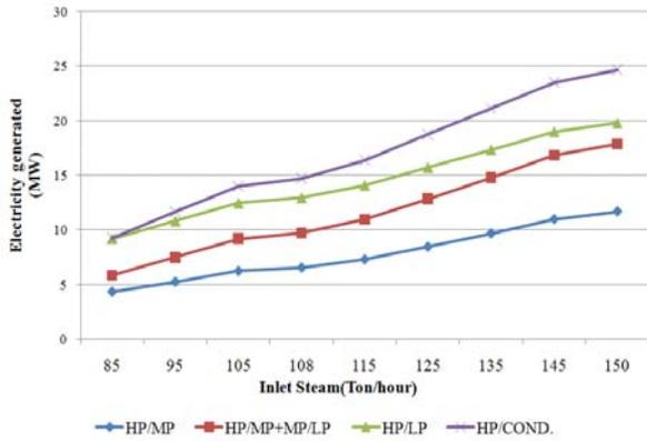
Fig. 3. Graph of changes in power generated in different technologies relative to steam mass
